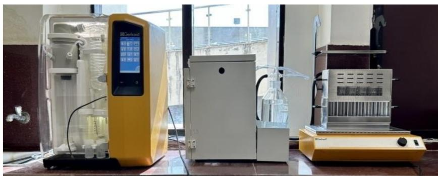
NITROGEN DISTILLATION AND DIGESTION WITH SCRUBBER
